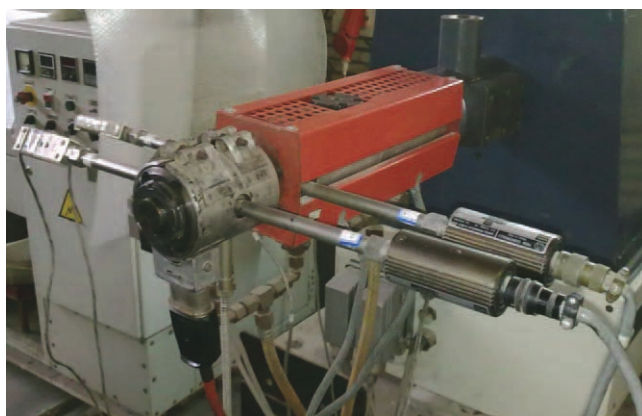
Figure 4 Laboratory extruder used for the extrusion process. [Color figure can be viewed in the online issue, which is available at wileyonlinelibrary.com .]
